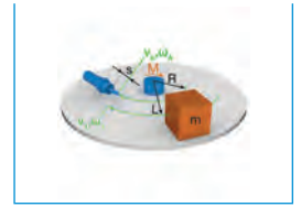
R7. Horizontally pivoting mass with frictional drive torque
