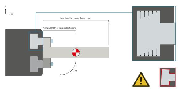
Mmax= 1/2 max. length of the gripper fingers \* max. dead weight, mounted gripper finger \* g
