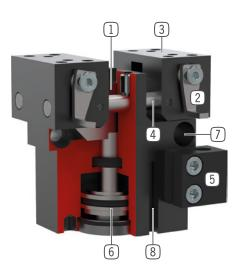
1 Wedge hook mechanism - synchronized the movement of the gripper jaws - high force transfer 2 Adjustable switch cam - for position sensing 3 Gripper jaw - individual gripper finger mounting 4 Roller slide - for low wear movement sequence 5 Mounting block - mounting for inductive proximity switch 6 Drive - double-acting pneumatic cylinder 7 Mounting and positioning - mounting possible from several sides for versatile positioning 8 Sensing slot
