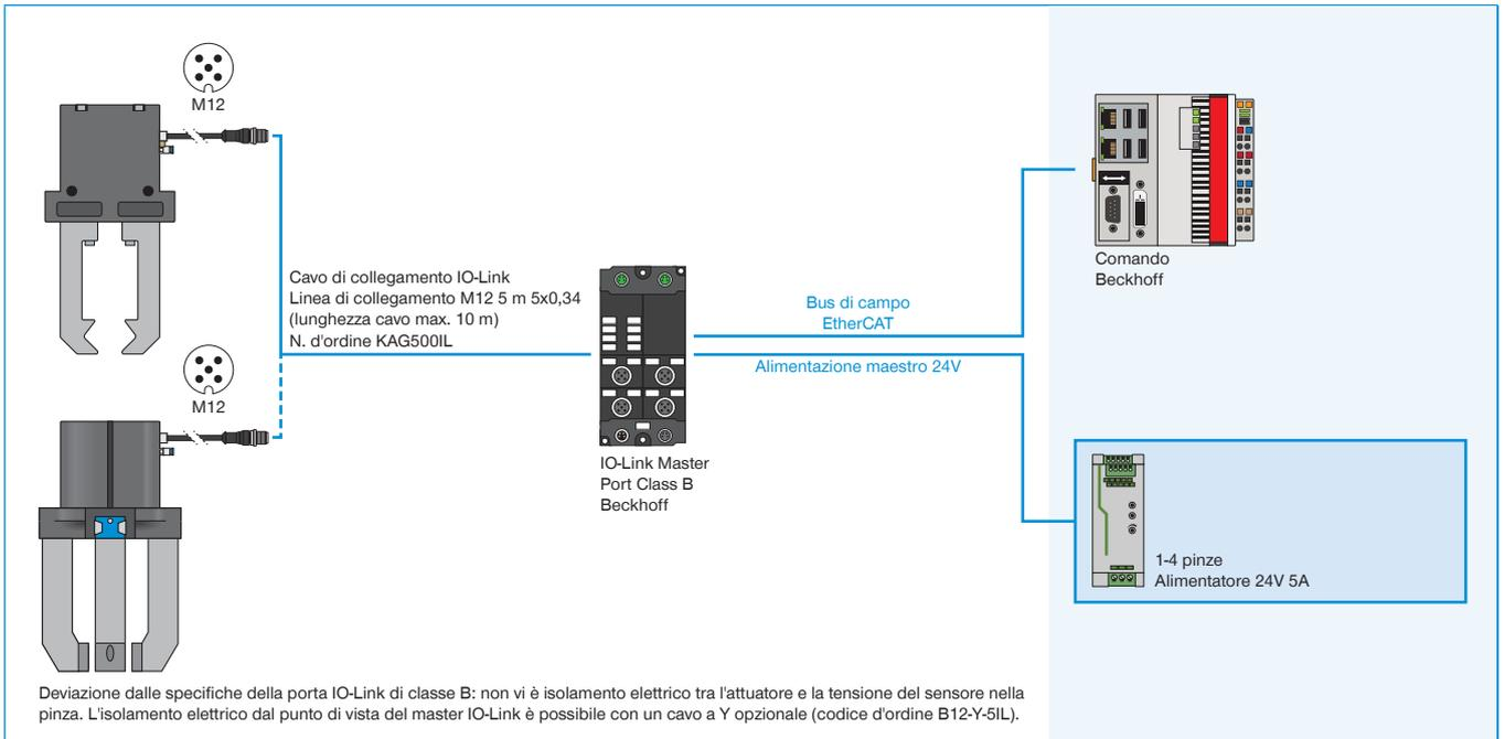
► GPP5000IL / GPD5000IL (IO-LINK) CABLAGGIO SU IO-LINK MASTER IP67 (SIEMENS)
