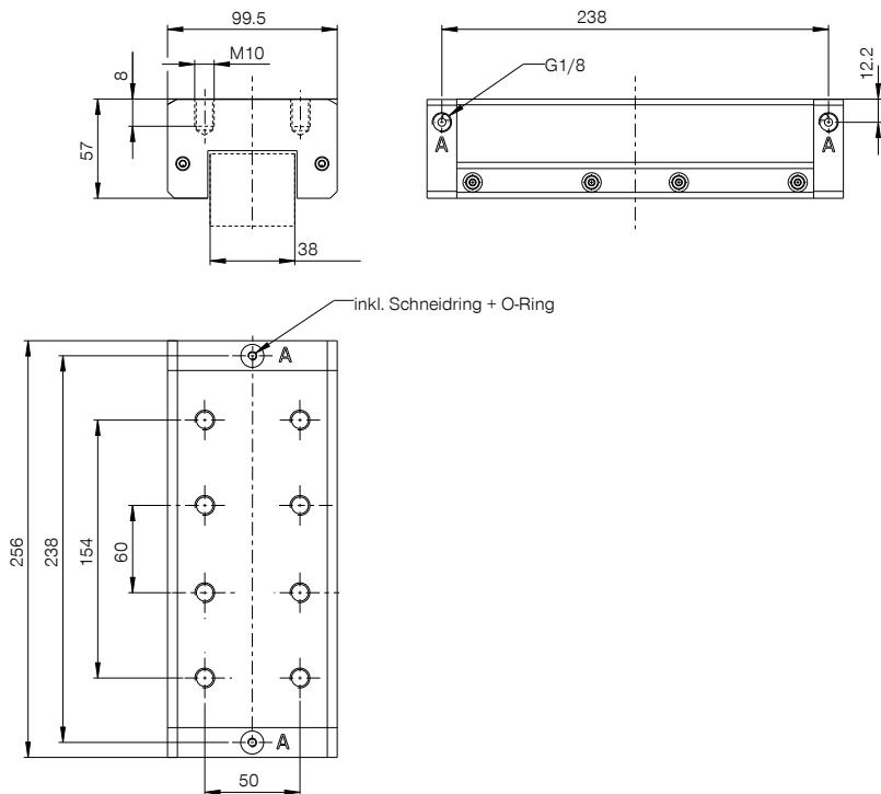
(A) Connection opening (both sides possible, only one connection necessary)
