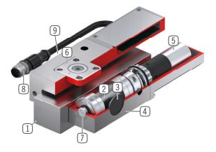
1 Profile rail guide - Available for all common profile rail guides 2 Eccentric gear - Power transmission between motor and clamping jaw 3 Clamping jaw - Pressed at the free surfaces of the profile rail guide (4) Housing 5 electric drive - For generating clamping force 6 Sliding block - For floating bearings 7 Emergency actuation - Manual opening possible in case of power supply failure 8 Electrical connecting cable - Control and power supply 9 Adjusting screw - Correction of the rail tolerance
