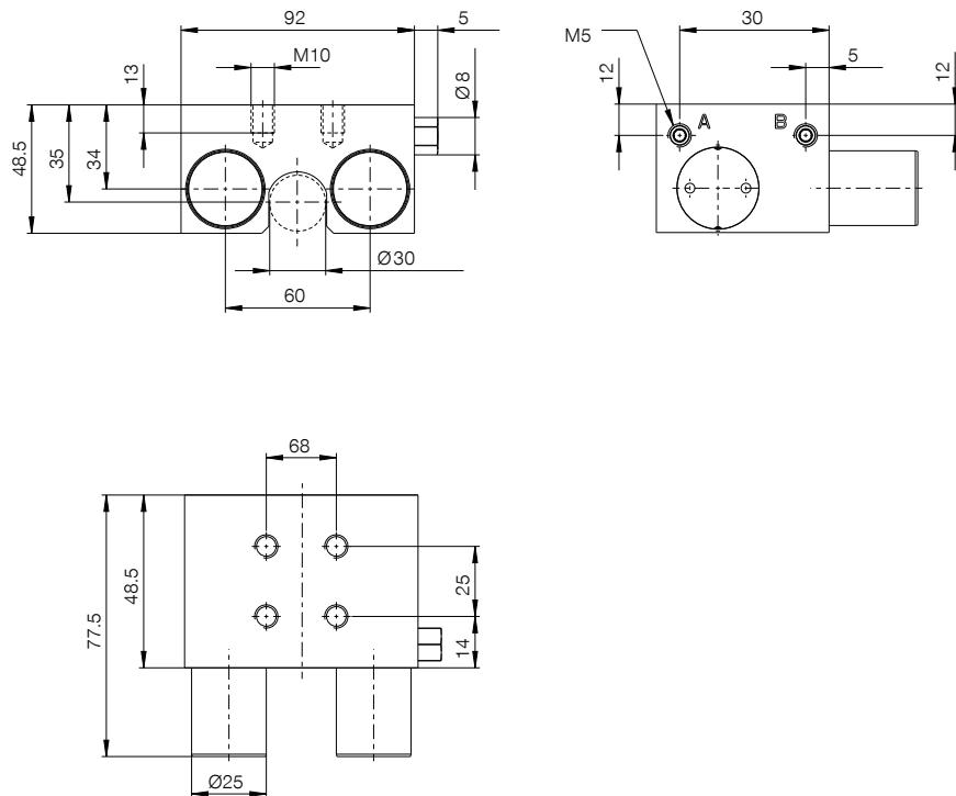
(A) Connection opening (both sides possible, only one connection necessary)
