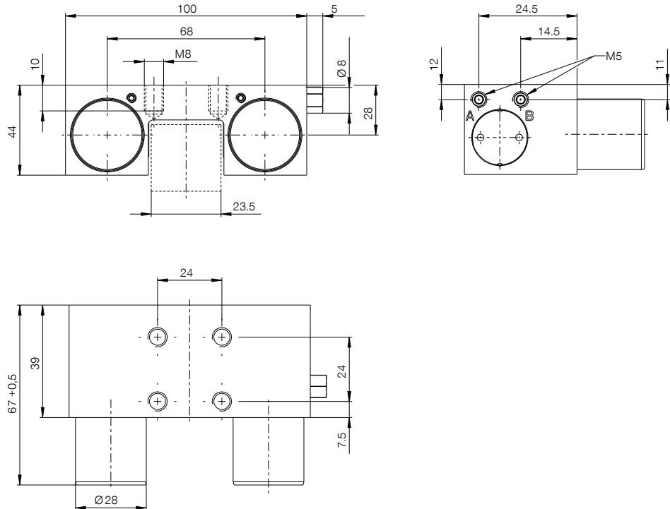
(A) Connection opening (both sides possible, only one connection necessary)
