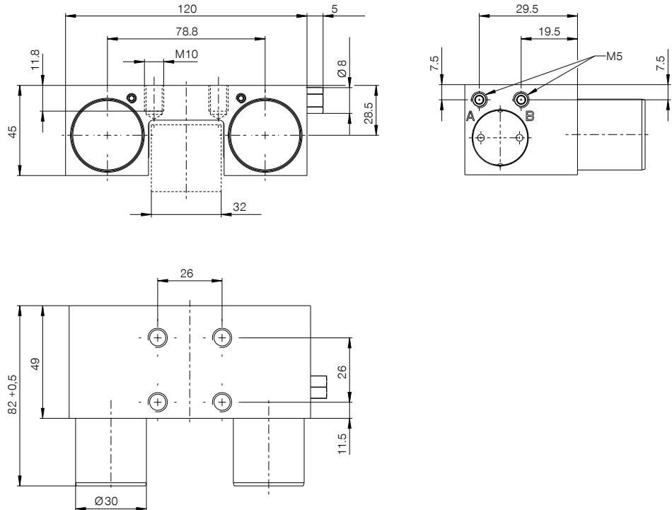
(A) Connection opening (both sides possible, only one connection necessary)
