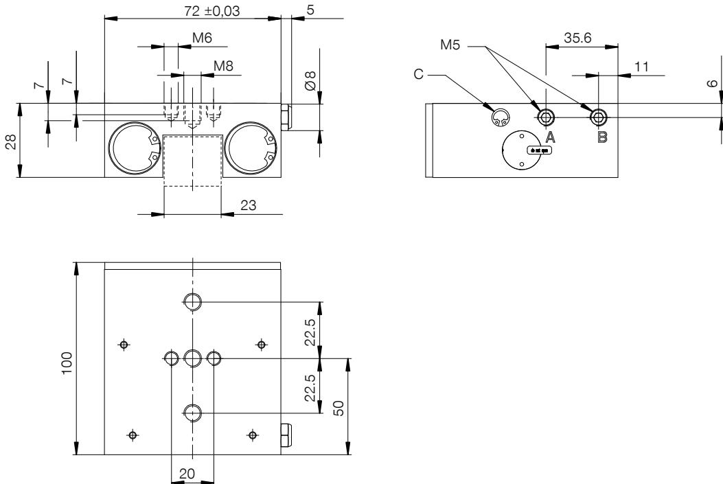
(A) Connection opening (both sides possible, only one connection necessary)
