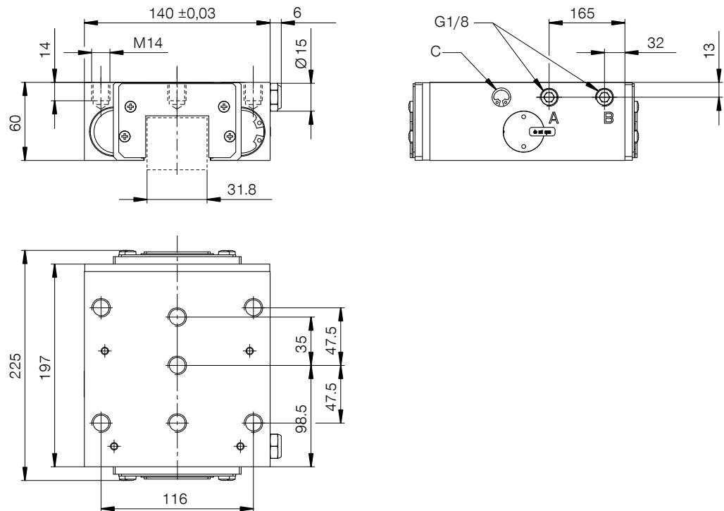
(A) Connection opening (both sides possible, only one connection necessary)
