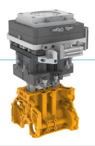
Loading and unloading machining centers with different types of 3-cylinder crankcases.
