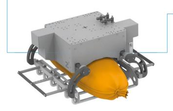
The Zimmer Group bag gripper is a one-of-a-kind end-of-arm system for handling bags filled with a wide variety of products. These include flour, fruit, vegetables, grain, fertilizer, chemicals, cement or numerous other products. A variety of bag materials can be used, such as paper, plastic, jute, cloth or fabric. A modular design enables the gripper to be expanded with additional functions such as intermediate layer gripper, pallet handling and much more.
