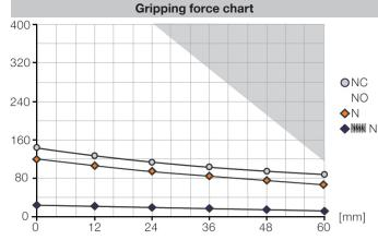
The chart shows the arithmetic total of the individual forces that occur on the gripper fingers, depending on the gripper finger length. The area shaded in gray marks the area where increased wear is to be expected.
