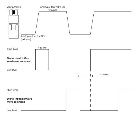
A movement in the desired direction occurs when the corresponding signal is at a high level. After a high level is detected, the gripper movement occurs until the gripping process ends.
