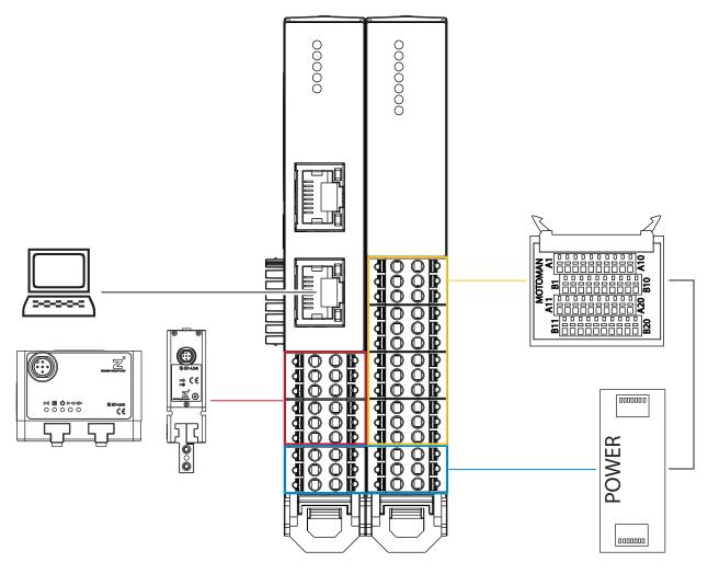
The standard wiring corresponds to the standard configuration in the Comfort App. If you do the standard wiring and keep the standard configuration in the Comfort App, your grippers will function with the robot.
