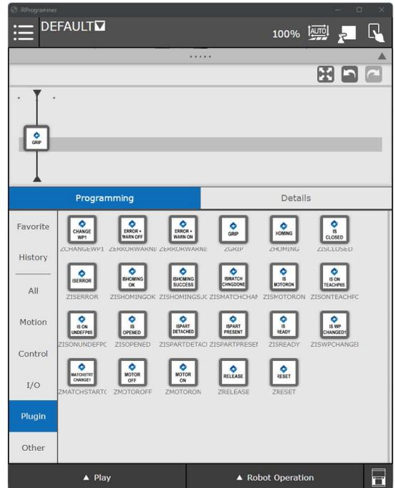
In this example, Register 2 receives the result of the command after executing the `ZISONTEACHPOS` command.
