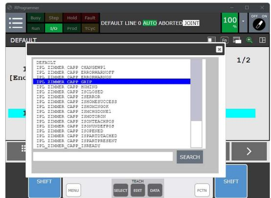
The `IPL_ZIMMER_CAPP_GRIP(1,7)` command queries the gripper 1 and register 7.
