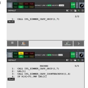
Line 1 and 3 address gripper 1 (gripper number).
