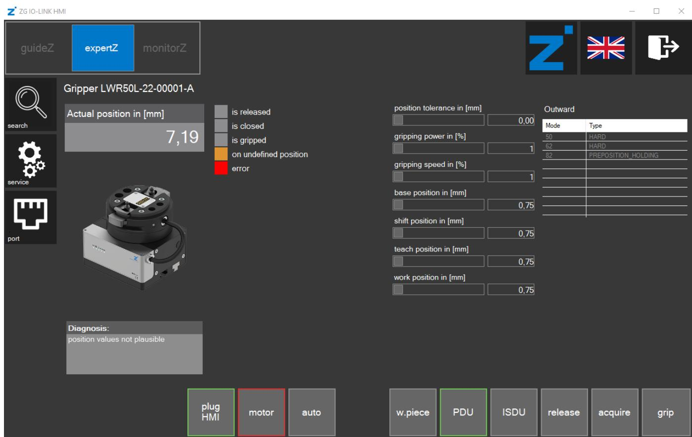
By default, the *fine tuning* setting is active. This is a view based on the parameters configured in the *guideZ* control level. You can optimize these parameters in this view.
