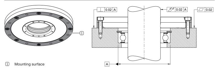
The product can be installed to the mounting piece from above via the pneumatic connection or from below via the mirrored drilling pattern.
