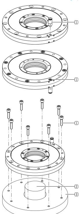
► Remove the screw fitting from the connection.
